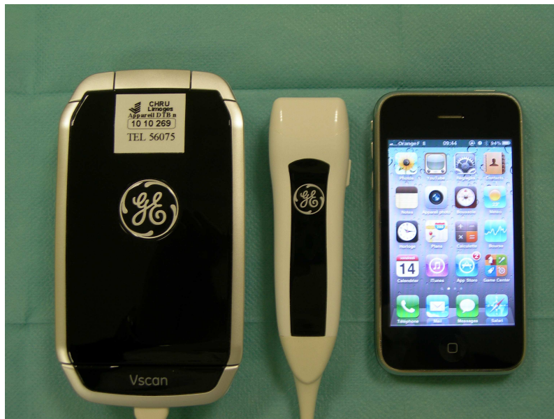
Figure 1 New generation miniaturized ultrasound system the size of a smartphone used in the current study.
