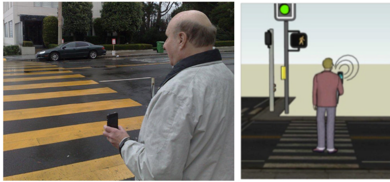
Figure 1. Crosswalk system for providing guidance to VI pedestrians at traffic intersections. (a) Blind user “scans“ the crosswalk by panning cell phone camera left and right, and system provides feedback to help user align him/herself to crosswalk before entering it. (b) Schematic shows that system announces to user when the Walk light is illuminated.
