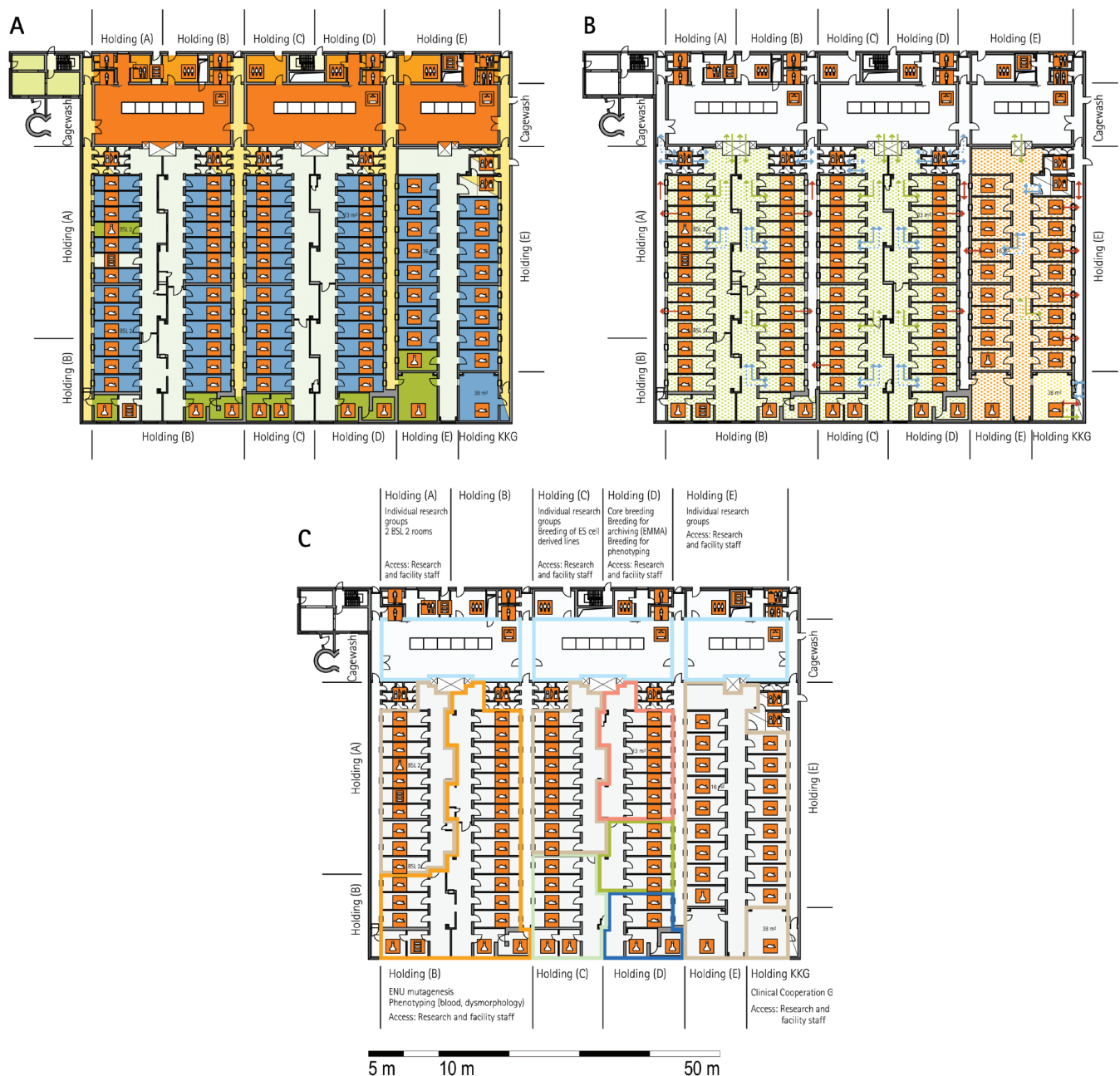
Figure 6. Schematic floor plans—facility 2, plan 2. (A) Zoning scheme. (B) Flow and hygiene levels scheme. (C) Functional unit scheme. For a description of the icons and colors used in the floor plans, see the legend to Figure 1.
