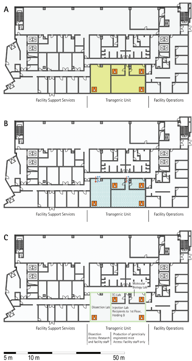
Figure 3. Schematic floor plans—facility 1, plan 3. (A) Zoning scheme. (B) Flow and hygiene levels scheme. (C) Functional unit scheme. For a description of the icons and colors used in the floor plans, see the legend to Figure 1.
