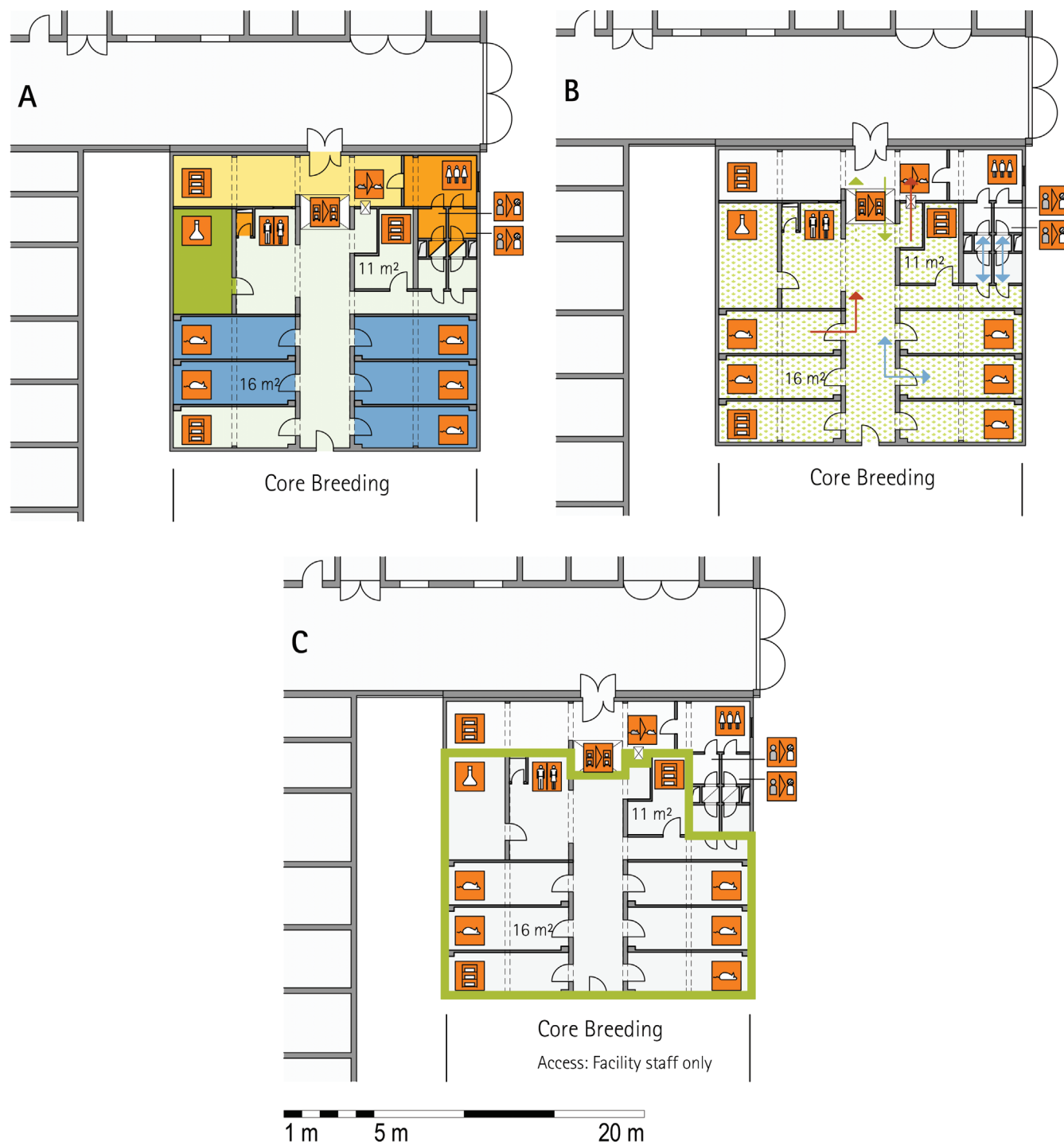
Figure 7. Schematic floor plans—facility 2, plan 3. (A) Zoning scheme. (B) Flow and hygiene levels scheme. (C) Functional unit scheme. For a description of the icons and colors used in the floor plans, see the legend to Figure 1.
