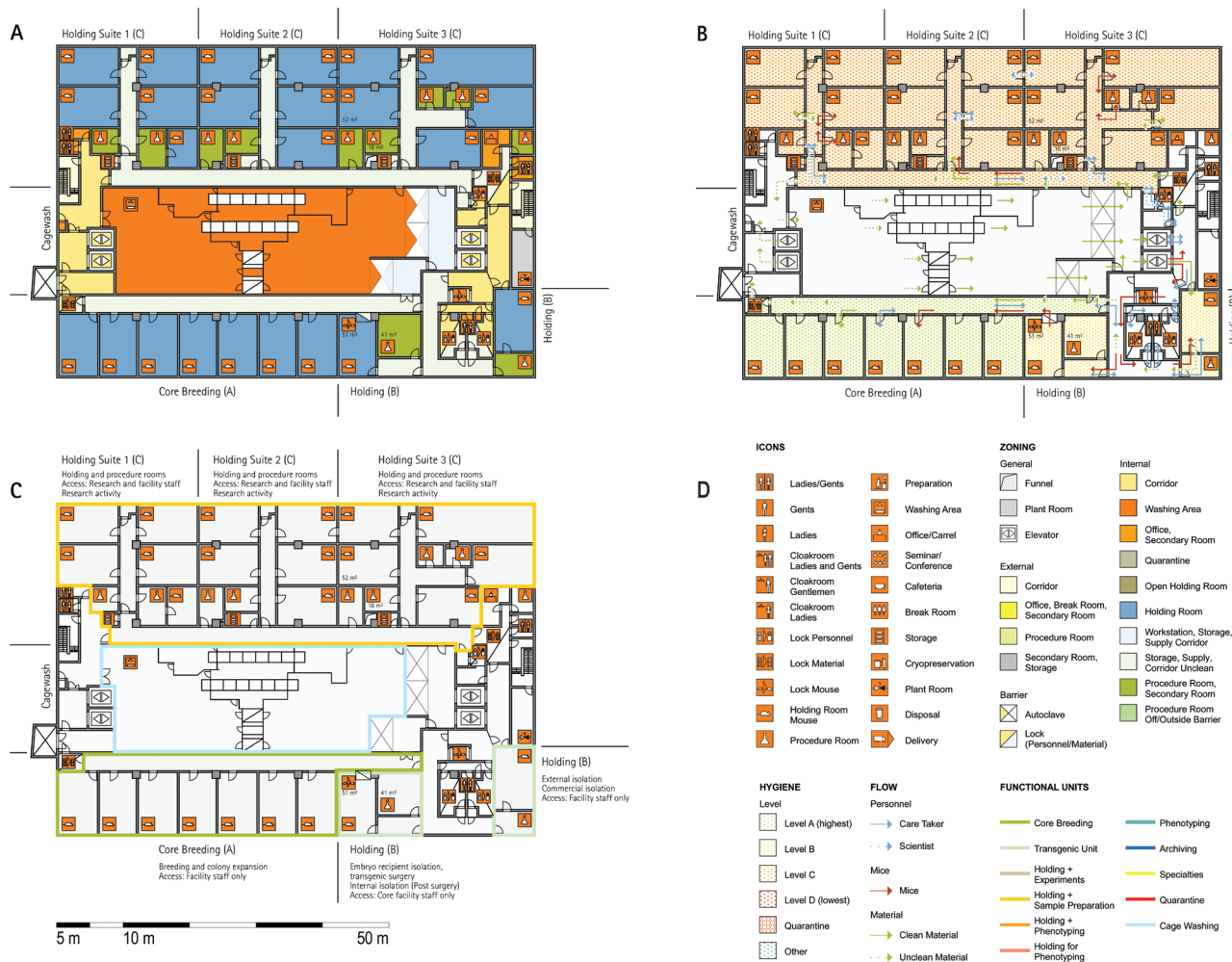
Figure 1. Schematic floor plans—facility 1, plan 1. Three types of schematic floor plans that outline the layout of the rooms and floors, the hygiene zones, and traffic flow were generated from the information collected at the visited facilities. (A) Zoning scheme. The zoning scheme shows the various functional types of rooms, which are represented by icons. In addition, color coding indicates areas outside and within the barrier as well as the various functional units. (B) Flow and hygiene levels scheme. The flow and hygiene levels scheme shows the flow of personnel (caretaker, scientists), mice, and material (clean and soiled) and the various hygiene levels. (C) Functional unit scheme. Details of the functional use of the various units and access of the facility staff and scientists are presented. (D) Description of the icons and colors used in the various floor plans.
