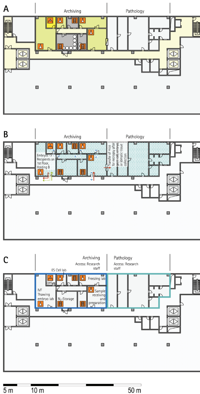
Figure 4. Schematic floor plans—facility 1, plan 4. (A) Zoning scheme. (B) Flow and hygiene levels scheme. (C) Functional unit scheme. For a description of the icons and colors used in the floor plans, see the legend to Figure 1.
