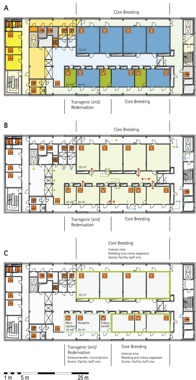
Figure 11. Schematic floor plans—facility 4, plan 2. (A) Zoning scheme. (B) Flow and hygiene levels scheme. (C) Functional unit scheme. For a description of the icons and colors used in the floor plans, see the legend to Figure 1.
