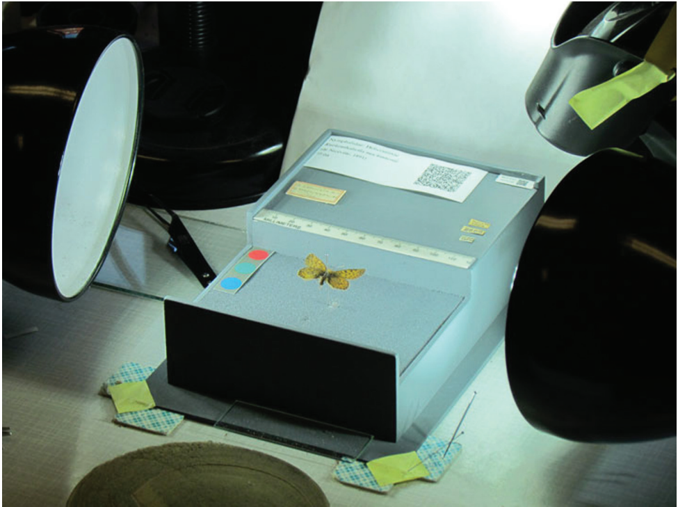
Figure 3. Custom specimen holder. Museum of Comparative Zoology (MCZ) Rhopalocera (Lepidoptera) Rapid Digitization Project.
