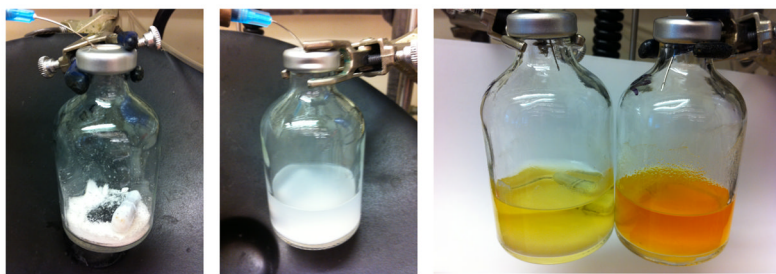
Figure 3. Color Change Indicating Completion of the Borylation Reaction: left to right: air stable solids during degassing; colorless reaction solution; completion of reaction [aryl chlorides turn yellow (left), aryl bromides turn orange (right)].
