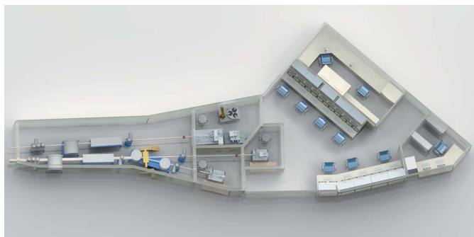
Figure 6 Three-dimensional drawing of the MX beamline optics (left) and experimental hutches (centre) as well as the experiment control room and sample preparation laboratory (upper right). Beamline order from top to bottom: BL14.1, BL14.2, BL14.3.
