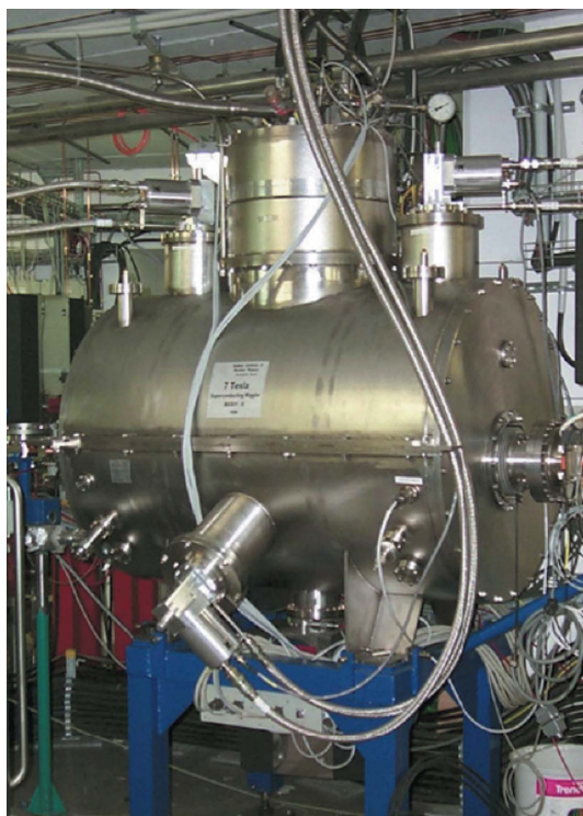
Figure 1 The 7T-WLS installed in the low- \beta section 14 of the BESSY II storage ring.
