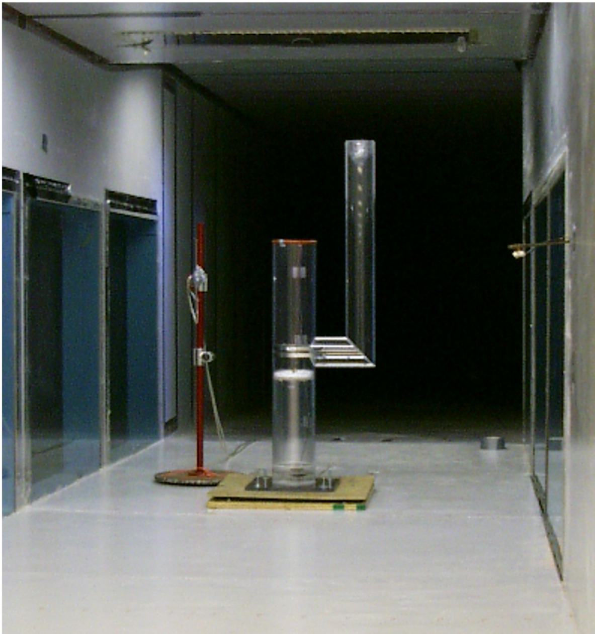
Figure 2. Scale model nest tree setup we used to calculate the h_c of unattended eggs. doi:10.1371/journal.pone.0041498.g002
