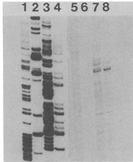
Figure 4. S_1 protection of a 5'-end labeled restriction fragment by total IMR 6 poly(A) + mRNA. After annealing and S_1 digestion (see Methods), the reaction products were analyzed on 5' / ° polyacrylamide-urea sequencing gel. Lanes 1-4 represent the dideoxy sequence (T,C,G,A) of a clone used as a size marker. Lanes 5,6; no mRNA controls. Lanes 7 and 8; IMR 6 mRNA. 2000 units of S_1 nuclease were used for the reactions analyzed in lanes 5 and 7. 3000 units of enzyme were used for the reactions analyzed in lanes 6 and 8.
