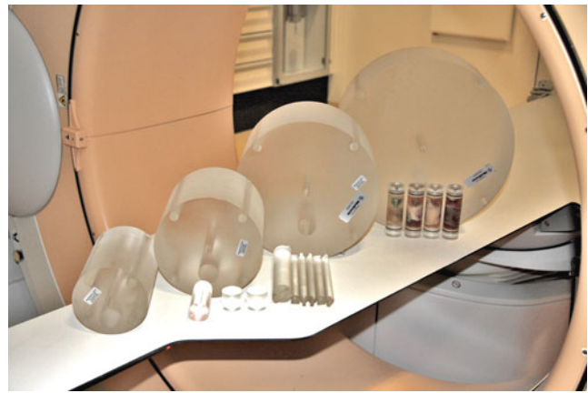
Fig. 1 Polymethyl-methacrylate (PMMA) phantoms with diameters 10–32 cm that were scanned together with inserts of bone specimens, solid PMMA rods and a tungsten wire
