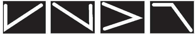
FIGURE 3. The above images are examples of path classes introduced for the mixed, single-angle tests. Each path here starts in the upper left corner. Each class is defined by the position of the turn relative to the start point and the general angle of the turn. Different members of a class are generated by horizontally, vertically, and diagonally flipping configurations.
