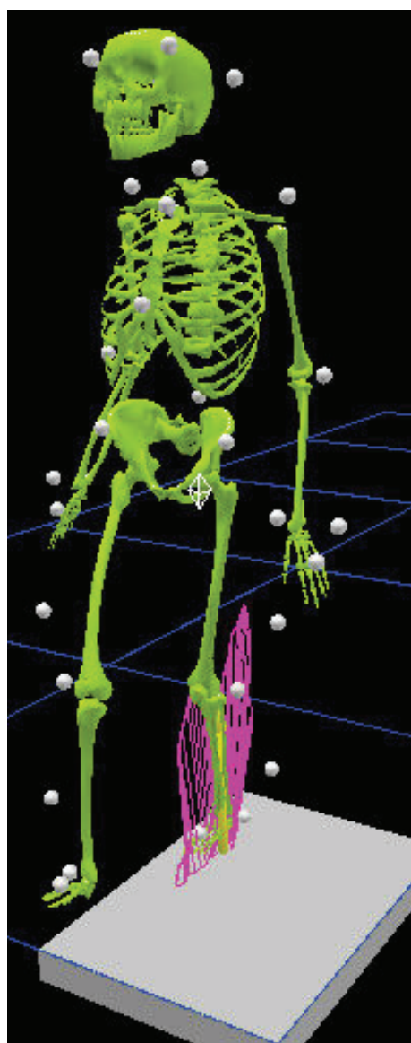
Figure 1 Biomechanical gait model (Plug-in-Gait, Vicon Motion Systems). 34 reflective markers (25 mm) were attached bilaterally by the same investigator (E.B.) onto the patient's skin over standardized bony landmarks (head, trunk, arms, pelvis, legs, and feet).
