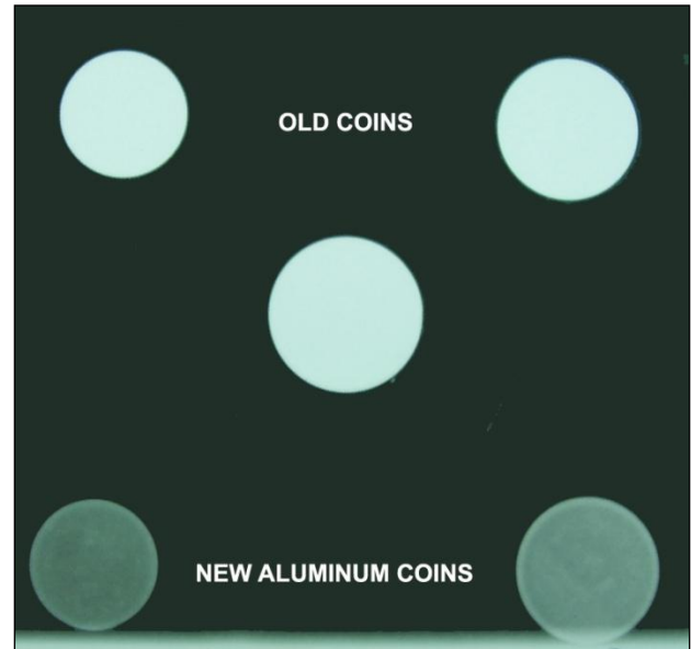
Figure 1: Old and new coins in comparison – radiologically.
