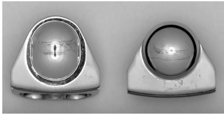
Figure 5. Micrograph of the superior (left) and inferior (right) endplates of a Prestige retrieved implant (2.3y in vivo ) showing a typical wear scar.
