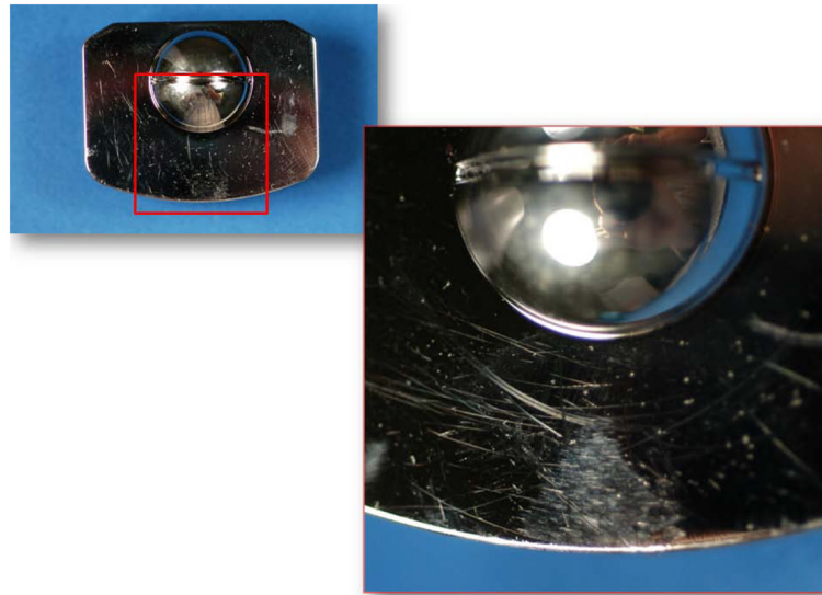
Figure 1. Micrograph of the superior (left) and inferior (right) endplates of a Maverick retrieved implant (1.5y in vivo) showing scratches and an area of impingement. (Color version of figure is available online.)
