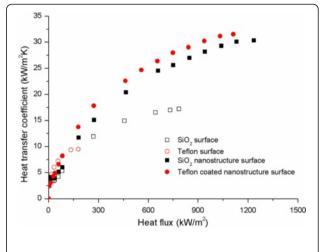
**Figure 4** Comparison of BHT coefficient on each of the different heating surface conditions.
