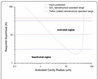
Figure 6 Comparison between Hsu's prediction [29] and actual activated range in real boiling condition.
