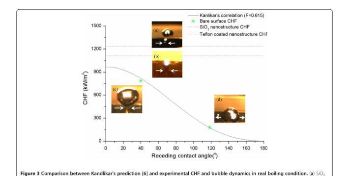
nanostructured surface, (**b**) Teflon-coated nanostructured surface, (**c**) SiO<sub>2</sub> bare surface, and (**d**) Teflon bare surface.
