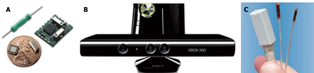
Figure 1 Various sensors which are commercially available [12] . A: Miniature magnetometers offer orientation and acceleration information, [Bertda Services (SEA) Pte. Ltd.]; B: Three-dimensional (3-D) range camera used in a widely commercial product; C: 3-D guidance system used in endoscopy devices (inition).
