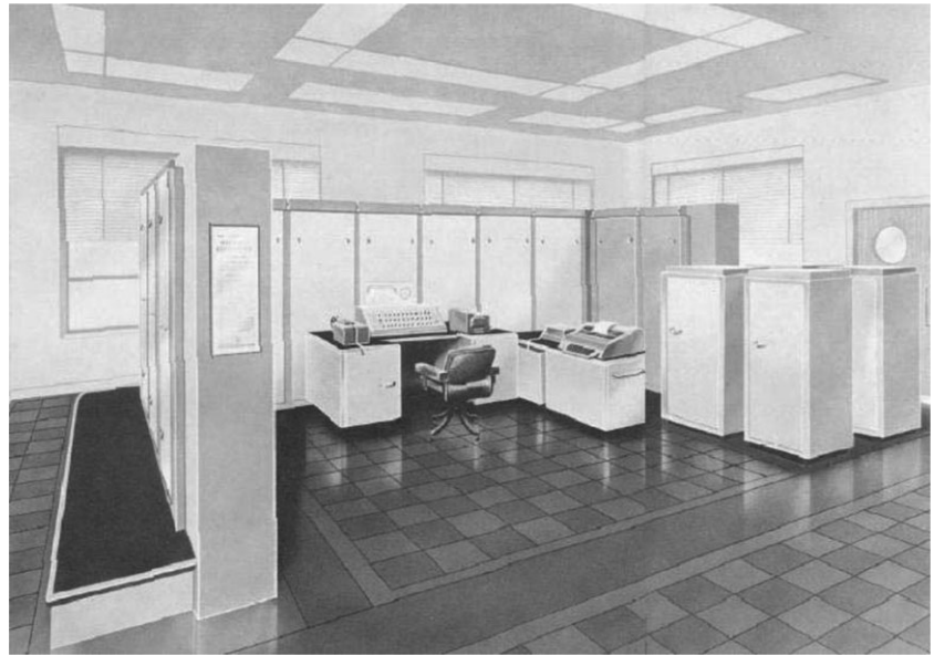
Figure 1. Schematic representation of the Ferranti Mercury computer, a valve-based machine
