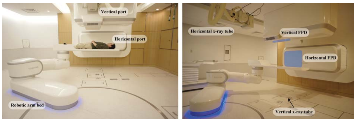
Fig. 1. Front view of the treatment room and installation of X-ray imaging devices [orthogonal X-ray tubes and flat panel detectors (FPDs)]
