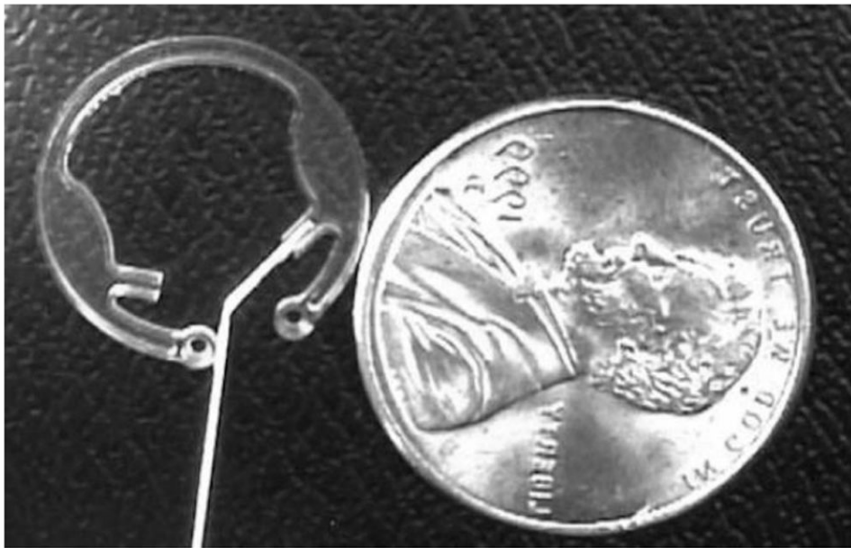
Fig 5. Reservoir-based, capsule drug ring with a 27 G cannula in the valve access port. Reproduced with permission from Fig. 3 in [54] (©2010 Elsevier).
