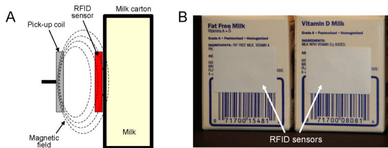
Figure 4. RFID sensor layout for demonstration of determination of milk freshness. (A) Schematic of sensor positioning onto a milk carton and sensor-response readout with a pick-up coil. (B) Photo of milk cartons with attached RFID sensors.
