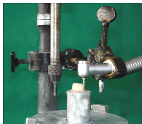
Fig. 2. Customized clamp to orient handpiece on the surveyor.
