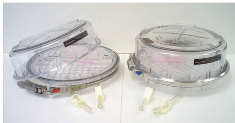
FIGURE 1: Cell-culture environmental chambers. Transwell plates were exposed to one of three levels of relative humidity: <20% (dry), 69% (noninterventional comparator), and >90% (HFNC) for 4 and 8 hours with 10 L/pm of room air at 37°C.
