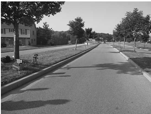
FIGURE 1. The un-signalized street used in our study to assess street-crossing decision-making ability. In the foreground on the left-hand side is one of the sensors that was used to calculate the vehicular gap times. The stool on the left-hand side is positioned by the crossing point where subjects made their street-crossing decisions.
