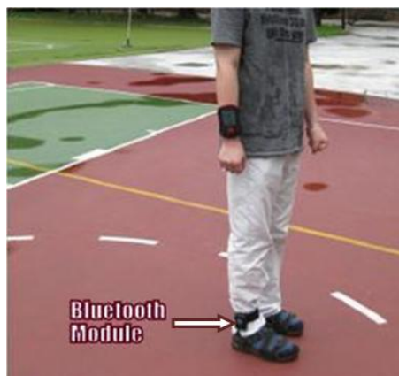
Figure 25. In-shoe plantar pressure measurement and analysis system based on fabric pressure sensing array [30].
