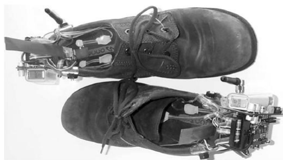
Figure 22. A wireless systems for gait and posture analysis based on pressure insoles and inertial measurement units [52].
