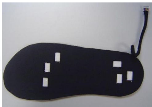
Figure 24. Fabric pressure sensing array indicating sensor placement [30].
