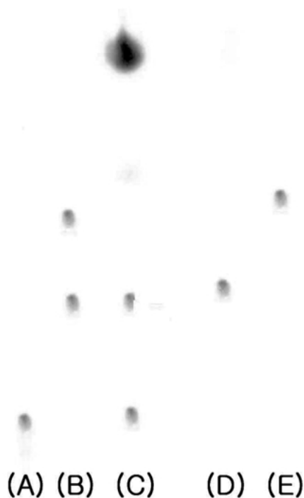
Figure 8. The result of TLC Analysis of the samples and a monomer 18, \beta -glycyrrhetic acid: glycyrrhizin (GL, standard)(A), enzymatically hydrolyzed GL (B), crude extract (C), Fraction 1 (D), 18, \beta -glycyrrhetic acid (GM, standard) (E).
