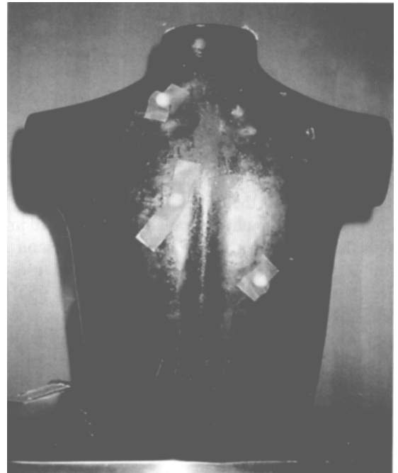
Fig 1. The anthropomorphic phantom with simulated lung nodules taped to different lung quadrants.
