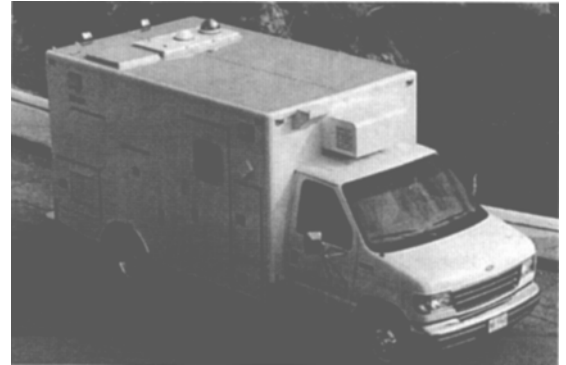
Fig 4. ACTS mobile terminal van. The Ka-band antenna is mounted on the left-rear corner of the roof. Reprinted with permission. 1
