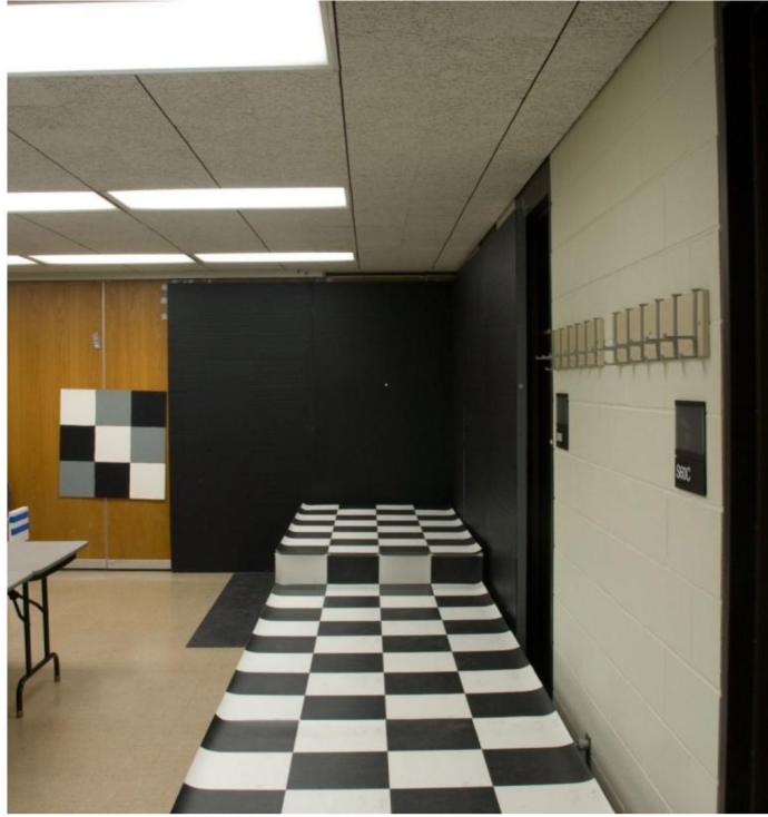
Figure 3. Photo of the test space, with the sidewalk and Step Up target covered by textured surfaces. The overhead lighting is also shown. A color version of this figure is available online at www.optvissci.com .
