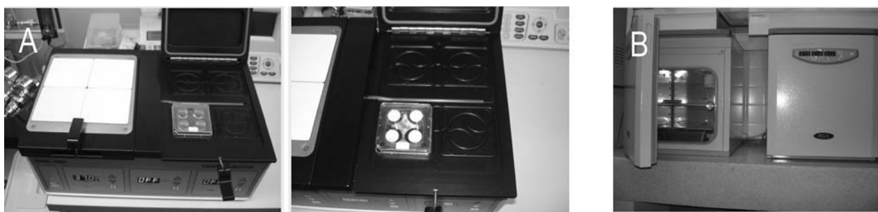
Fig. 1 Photograph of top-load mini-incubator and front-load conventional incubator: (A) top-load mini-incubator; (B) front-load conventional incubator
