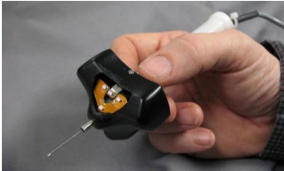
Fig. 7. Micron handpiece, showing tool and position sensor LEDs (visible through the window in the housing).
