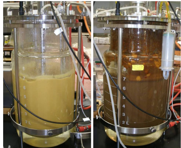
Fig. 2 Culturing H. bacteriophora in liquid media: (Left) Fermentor prior to Photorhabdus inoculation. (Right) After 21 days of rearing nematodes
