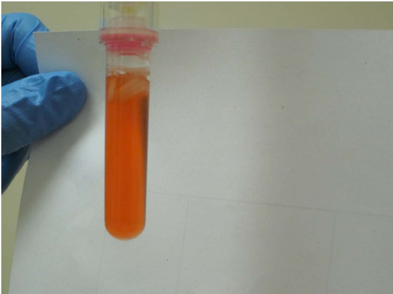
Figure 3. Example of a SmokeScreen positive test result. Original urine colour (no colour change) = negative test result. Dark blue-purple IsoScreen test = positive test result. Orange-pink SmokeScreen test = positive test result. Any other colour change = indeterminate test result. doi:10.1371/journal.pone.0045913.g003
