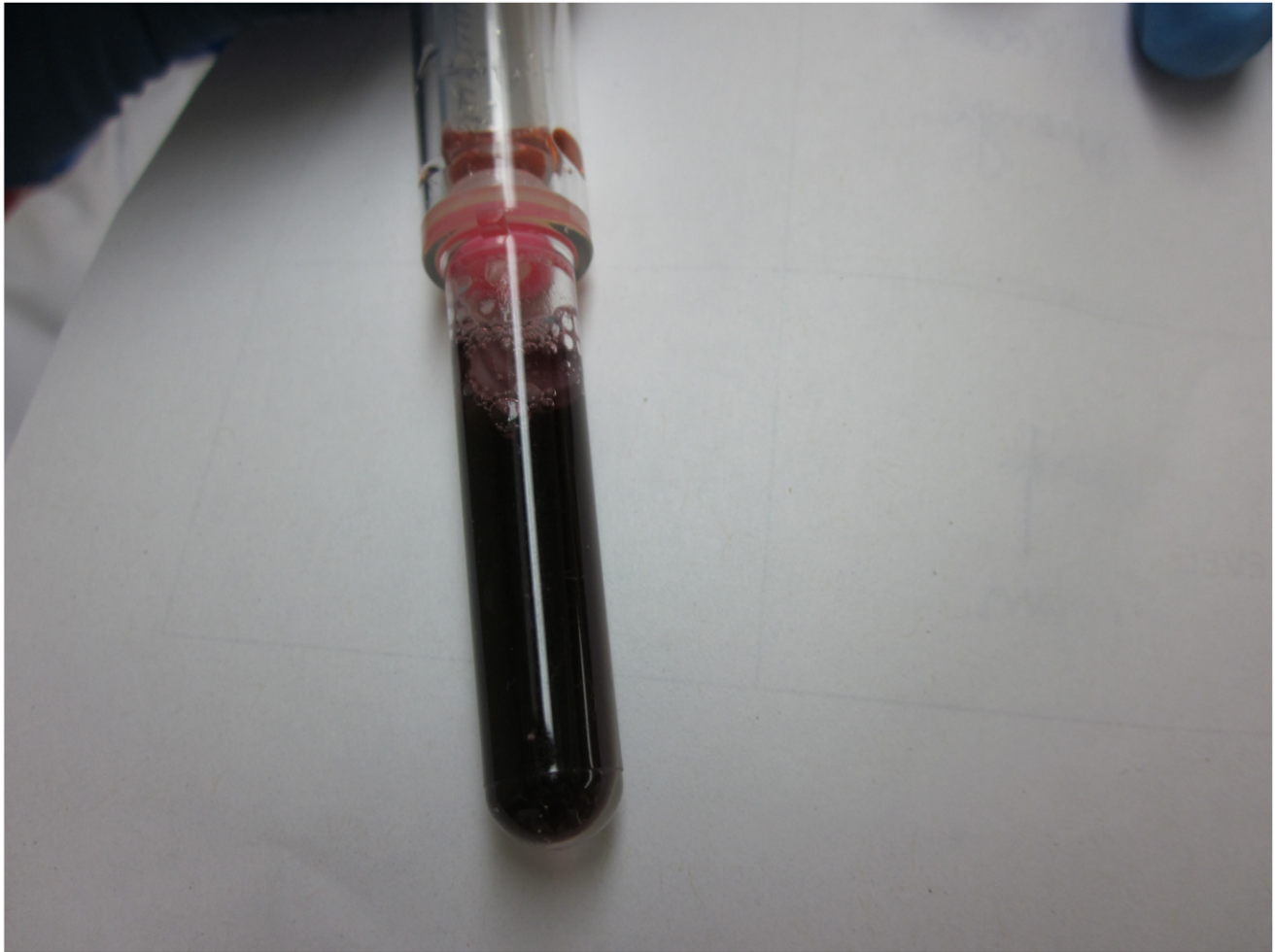
Figure 5. Example of an indeterminate SmokeScreen result. Original urine colour (no colour change) = negative test result. Dark blue-purple IsoScreen test = positive test result. Orange-pink SmokeScreen test = positive test result. Dark blue SmokeScreen test (not orange-pink) = indeterminate test result.
