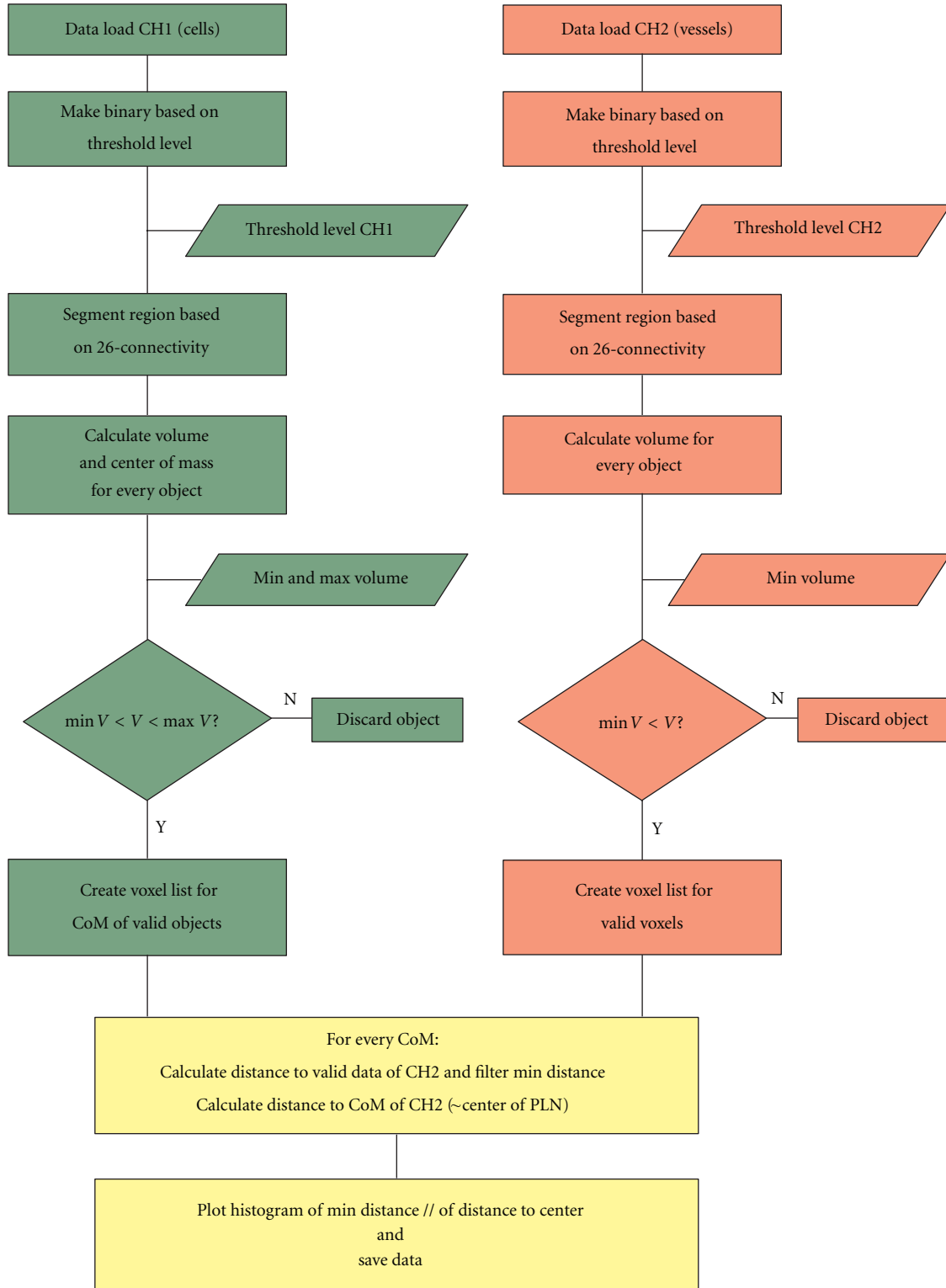
FIGURE 2: Flow diagram of the quantification algorithm. In the left path (green) dendritic cells are processed, in the right path (red), the vasculature data. The actual nearest neighbor search is done in the unified path (yellow). Abbreviations: center of mass (CoM), volume ( V ), peripheral lymph node (PLN).
