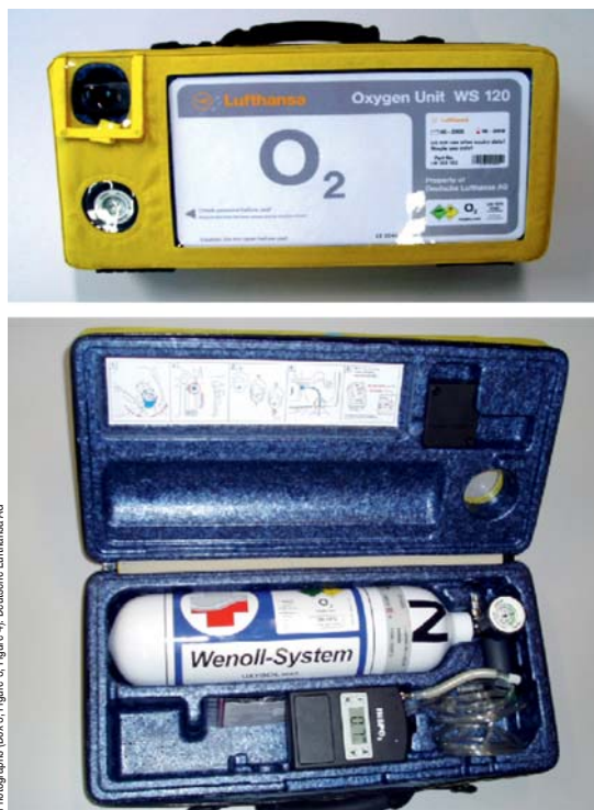
Figure 4: Supplemental oxygen: a 2 L carbon-composite cylinder at a pressure of 300 bar. Oxygen flows of 1.2 to 5.2 L/min can be achieved for 10 to 20 hours with the aid of an electronic valve (actuated by the drop in pressure during inspiration). This system is used by Lufthansa, Swiss, Air France, and other airlines. A pulse oximeter is incorporated in the shockproof hard-shell case
