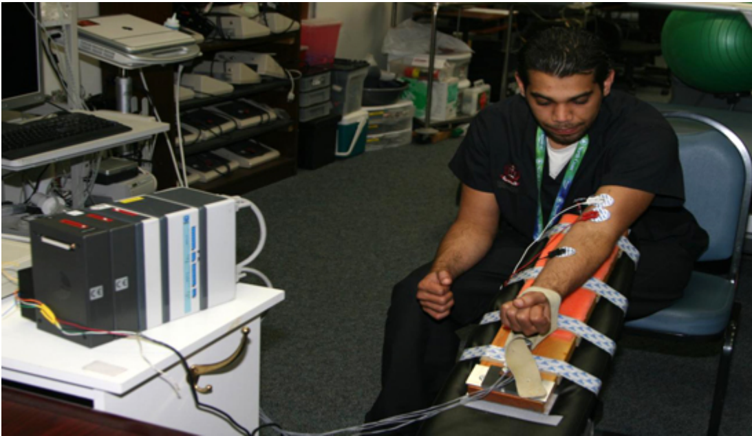
Figure 11. A typical subject exerting force on the strain gauge device.
