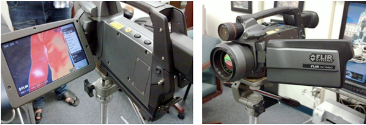
Figure 8. The IR thermal camera used for this investigation (FLIR 660).
