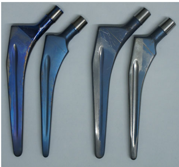
Fig. 4 Retrieved Titan® stems show variations in proximal stem geometry and color between groups. Stems shown from left to right are Group A lateralized, Group A standard, Group C lateralized, and Group C standard.
