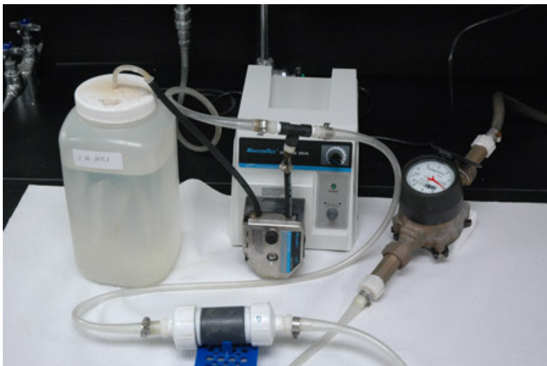
Figure 2. Glass wool filtration with acid injection by peristaltic pump. Note the "T" connector where the pump tubing introduces acid into the sample line between the water tap and glass wool filter. pH adjustment is necessary only if the water sampled has a pH > 7.5.
