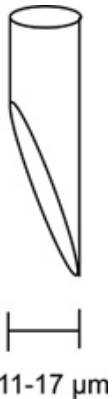
Figure 3. Beveled injection micropipette. A diagram of a properly beveled micropipette is shown here. The electrode opening should be beveled at a 45 degree angle and have an opening between 11 to 17 \mu\text{m} . A proper beveled injection micropipette is crucial for a smooth injection with minimal damage to the fly.
