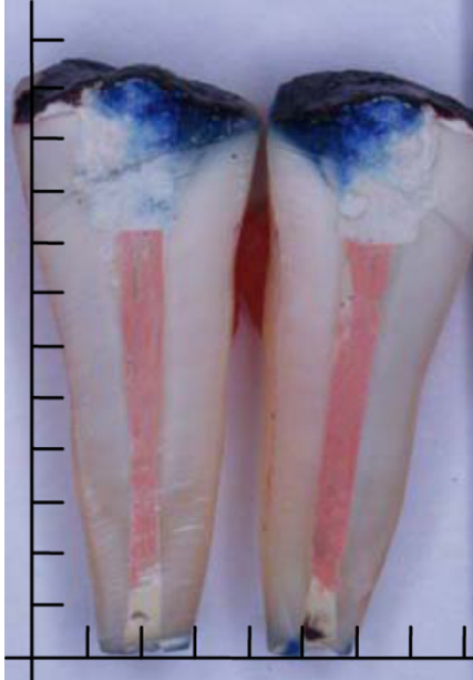
Figure 1. Photograph of a sectioned tooth after dye penetration (the distance between two lines represents 2 mm)
