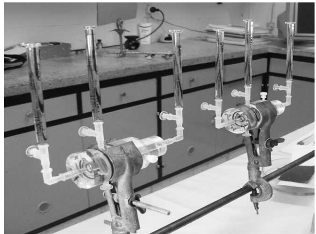
FIGURE 3. Photograph of two chambers set up during an open-circuit experiment; that is, the T-connectors between the glass Hamilton syringes and the Lucite chamber were closed with plugs (seen at a right angle to the glass capillaries). For short-circuit experiments, the plugs were removed and Ag/AgCl electrodes were inserted into the connectors (not shown).
