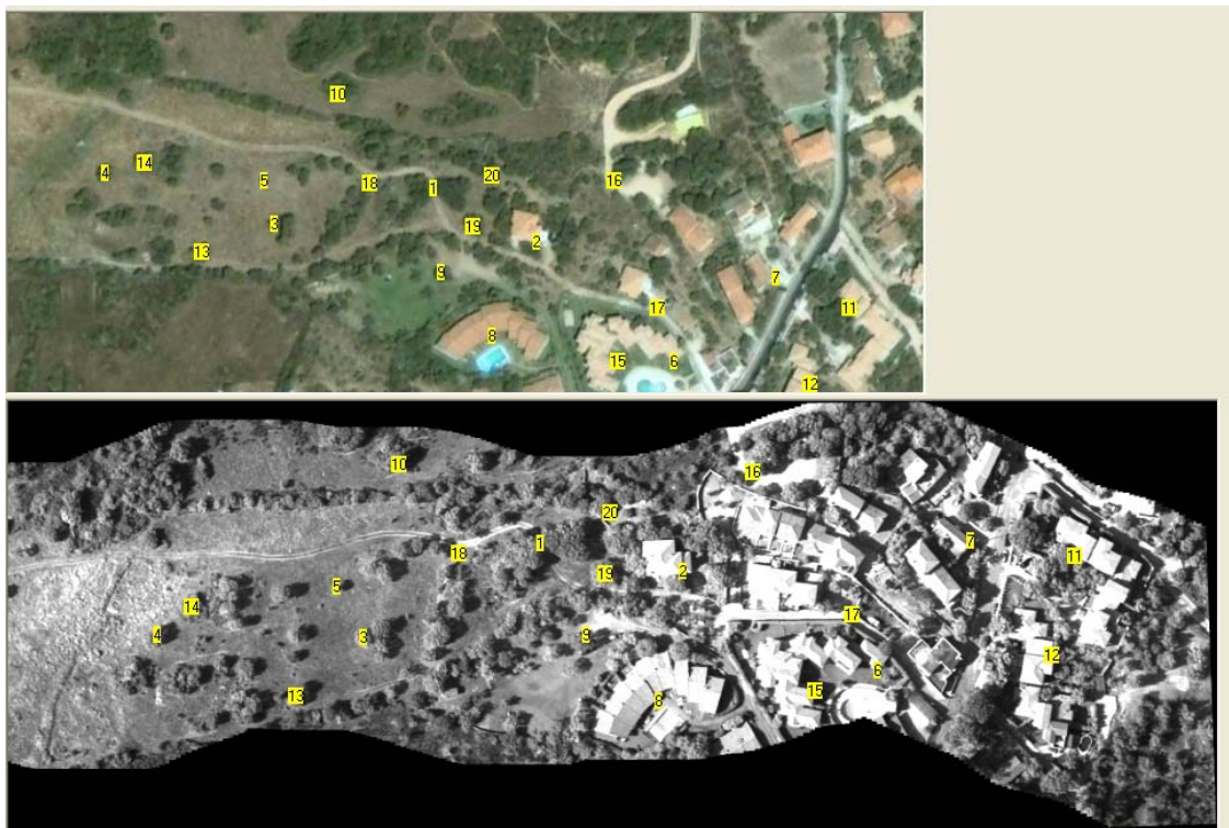
Figure 14. Map extracted from Google Earth employed for georeferencing both the mosaic and the images of the hyperspectral cube. The points employed for the geometric transformation are shown in white.
