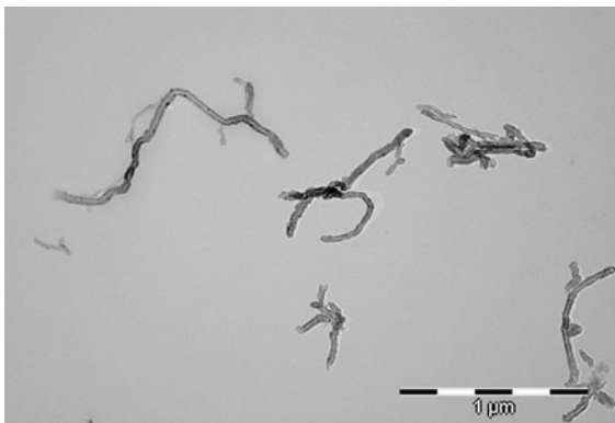
Fig. 7 TEM photomicrograph of MWCNT after chemical functionalisation (MWCNT-F)
