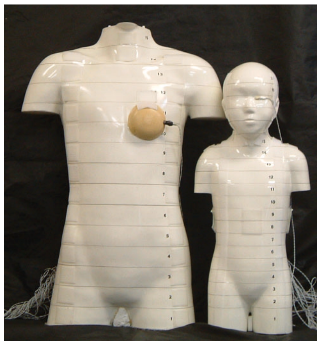
Figure 1. Adult phantom (left) and paediatric phantom (right) dosimetry systems. Seen with the phantoms are twisted carbon-fibre cables derived from photodiode dosimeters embedded within the phantoms.
