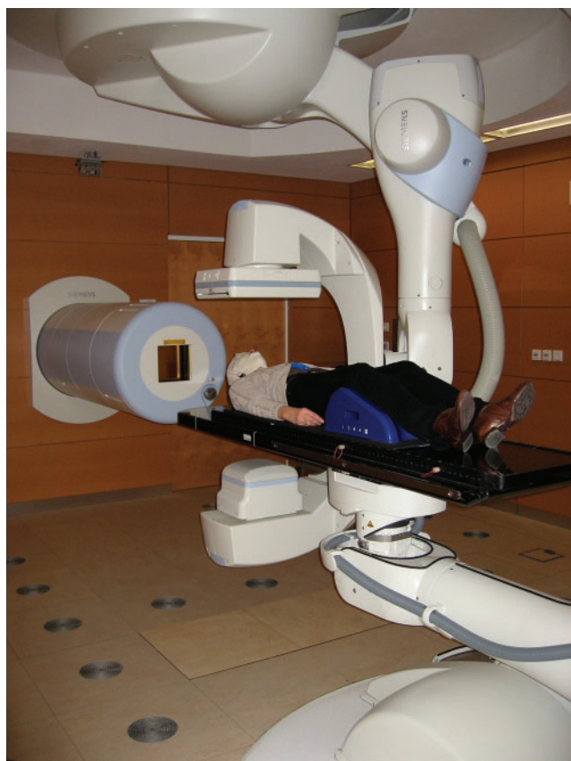
Figure 2. The Heidelberg Heavy Ion Centre’s horizontal treatment room has facilities for robotically controlled patient positioning and imaging.
