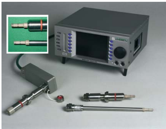
Figure 2. The Biomass Monitor with the variety of probes used in manufacturing processes.
