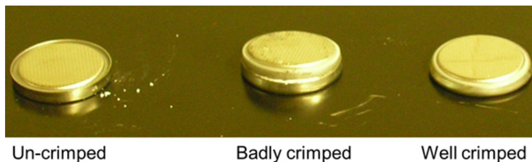
Figure 5. Comparison of a well crimped coin cell and a badly crimped coin cell, along with an un-crimped cell. Typically, a badly crimped coin cell splits open after a few hours in ambient due to the swelling of lithium foil after reaction with moisture.
