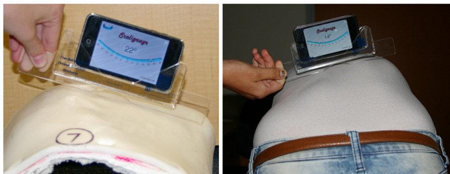
Figure 3 Measurement of the rib hump on a (a) plaster model and a (b) scoliosis patient, using the iPhone and Scoliguage software in combination with the acrylic sleeve to reflect the dimensions of the traditional Scoliometer.
