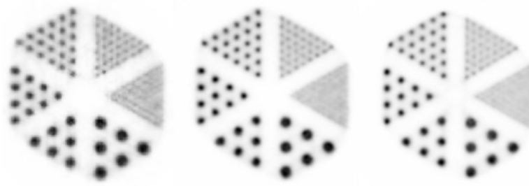
Figure 10. Comparison of the simulated 18 F rods in water phantom reconstructed with the ray-tracing OSEM 2D (left), iso-Gaussian (middle) and LOR-PDF (right) protocols.
