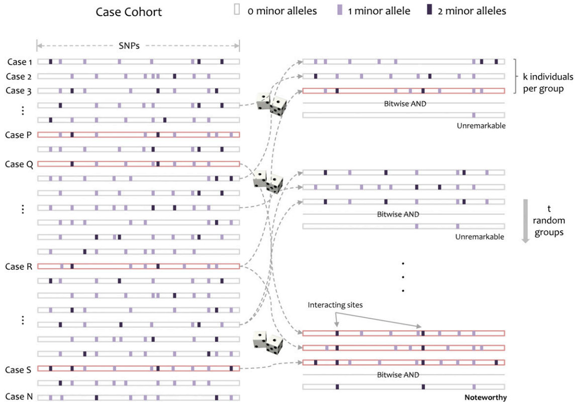
Figure 1. Group sampling. A cohort of N cases is shown on the left, where the cases outlined in red— P , Q , R , and S —harbor an interacting pair of recessive variables. In other words, more cases carry the recessive–recessive combination than would be expected by chance, given the marginal frequencies of each recessive allele. By repeatedly drawing random groups of k cases (here k=3 ), we are guaranteed to have drawn at least one group of individuals that carries both the variables in t attempts with probability \geq (1 - \beta) . These variables (and others) are quickly determined by a bitwise-AND operation between the group of cases. Then, all pairs of cocarried variables are enumerated and tested against the stage 1 null hypothesis (case-only analysis). Rejected combinations are shortlisted and followed up in stage 2 (case vs. control analysis), where an interaction is identified.
