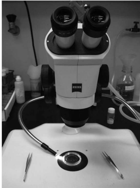
Fig. 3. Stereo microscope and light setup for larval dissections. The glass dish is under the microscope with the light source to the left side . Each hand will hold a pair of forceps during dissection.
