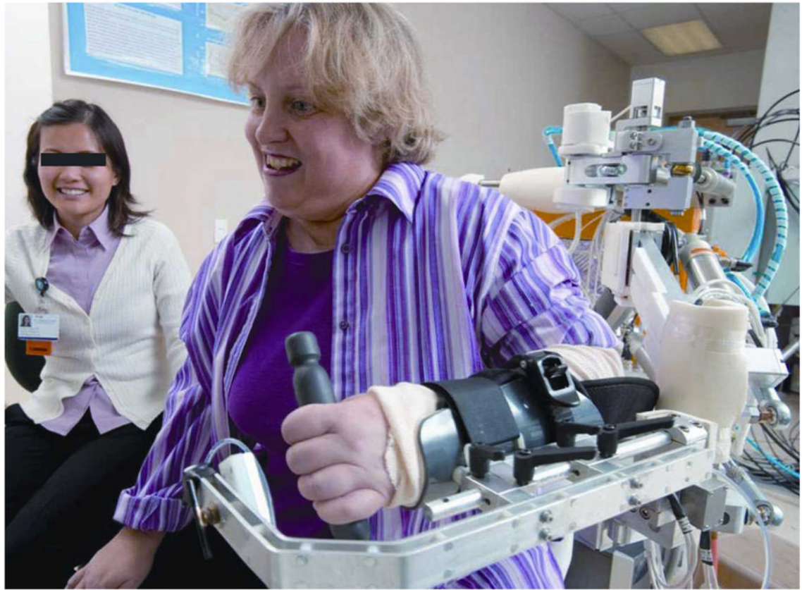
Figure 1. Pneu-WREX is a four degree-of-freedom pneumatically actuated upper extremity orthosis for robot-aided movement training. The user can move her hand in 3D space, and use the grip sensor to grasp and release virtual objects on the computer screen.
